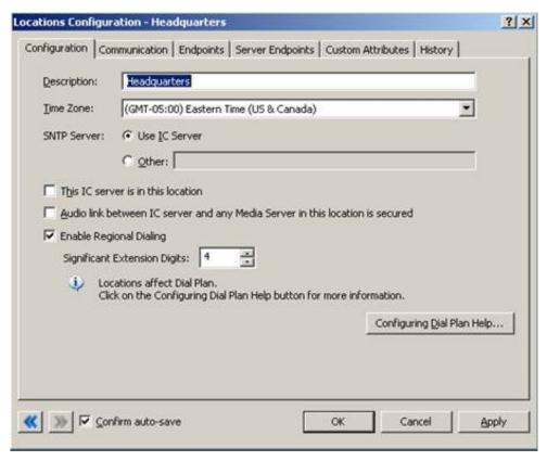
If you are configuring the location for the CIC server, select the This CIC server is in this location check box on the Configuration tab.
