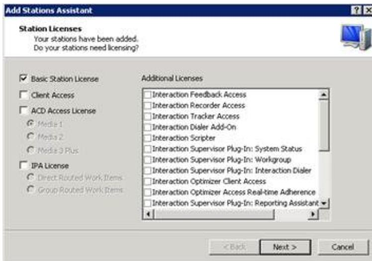
We recommend that you assign a Basic Station license to the stations. The Basic Station license allows station audio for a phone device or the soft phone on a client workstation.
