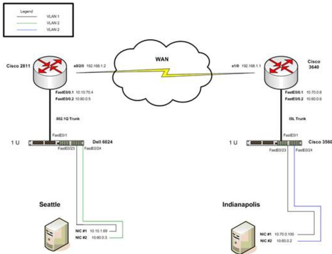
This diagram illustrates a sample WAN switchover configuration for one side of the network. The same configuration is required for the other side of the network. Configure the following components:
