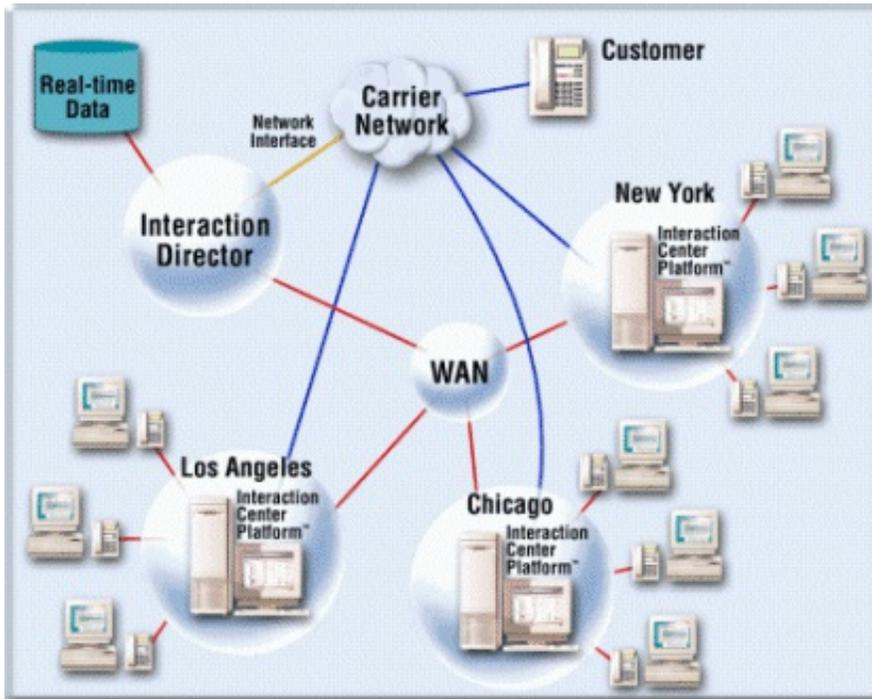
You can think of pre-call routing as "carrier-based routing" since routing decisions occur before the call connects and are based on signaling information from the carrier network.
