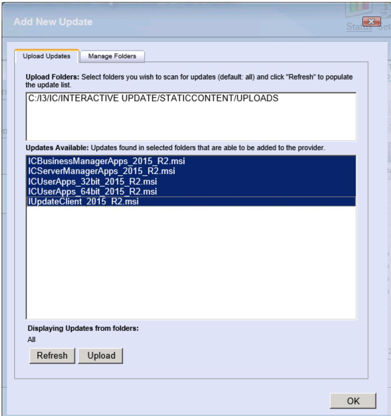
5. Click **Upload** to upload the contents of the selected update directory to the local provider. An **Uploading** progress bar appears until the upload is complete.
