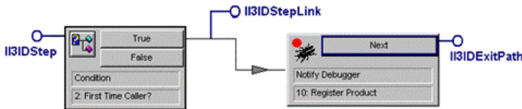
The **IISIDStep**, **IISIDStepLink**, and **IISIDExitPath** interfaces wrapper tool steps, exit paths, and linkages between steps.
