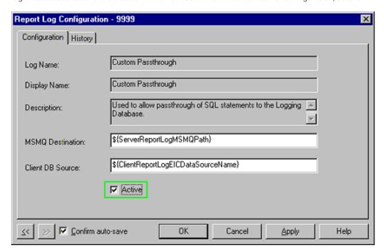
Use this tool to modify data using an ODBC SQL statement or statements. The ODBC distinction indicates that this tool allows escape sequences. CIC assumes this statement will run on the same server and on the same database. While the database utilities can be used to modify data as well, we recommend using the Logging Custom Passthrough (LCP) tool when asynchronous writing to a database is desired.
